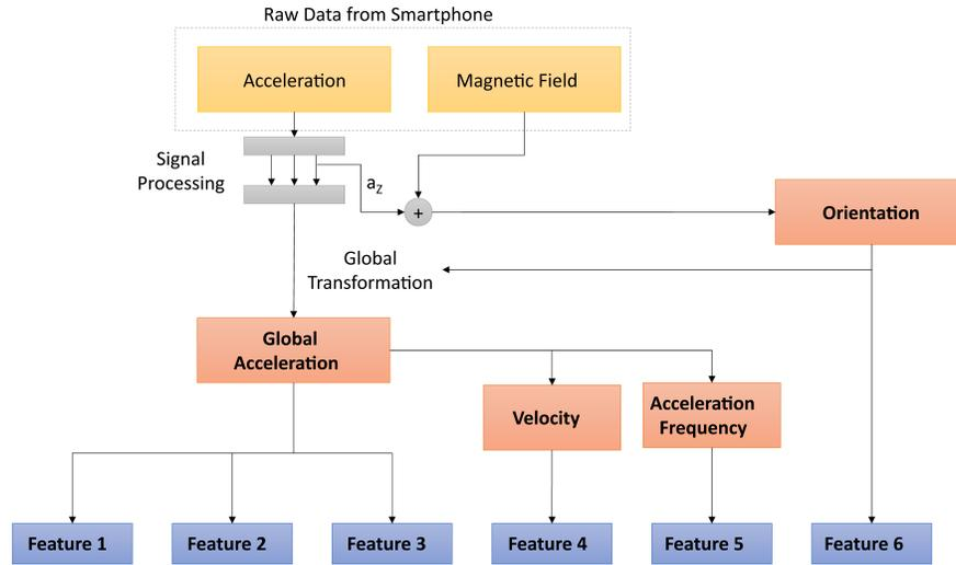
**Fig. 9.** Flowchart for feature extraction from sensor data
