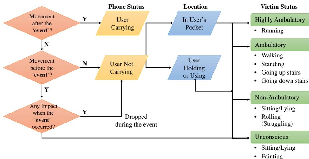
Fig. 6. Flowchart for determining the status using PVAS
