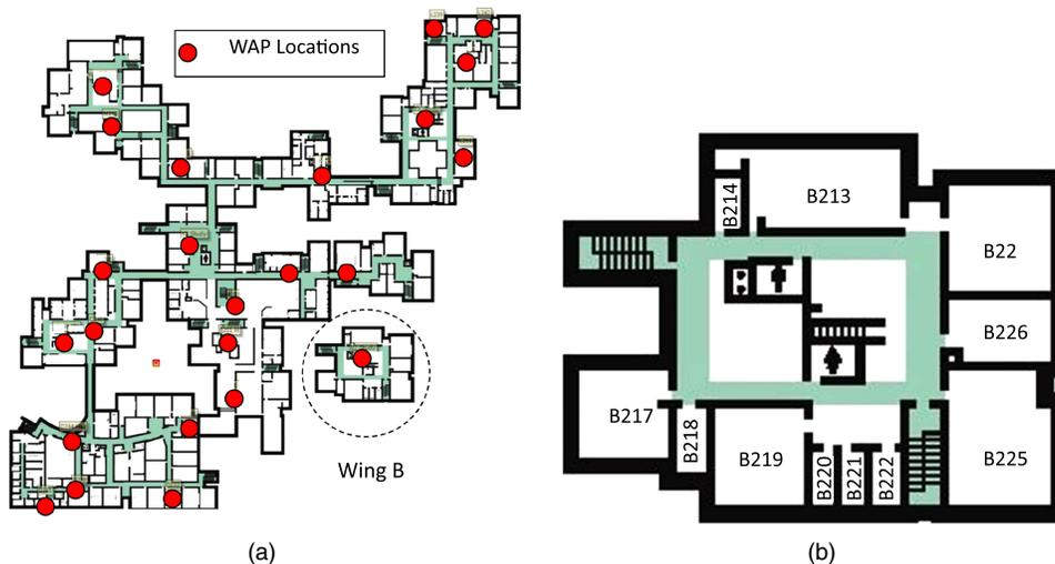
**Fig. 14.** Floor plan and location of WAPs for (a) 2nd floor of Parkland College; (b) for Wing B
