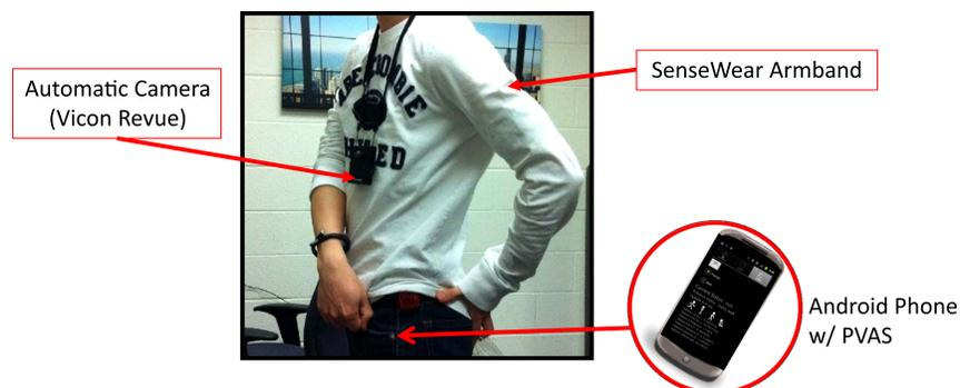
Fig. 19. Configuration of equipment for real-time monitoring test (image by Robin E. Kim)
