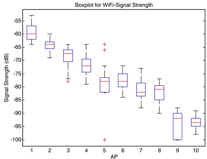
**Fig. 3.** Box-and-Whisker plot illustrating RSSI variability over a 100 s recording epoch for 10 different wireless access points detectable from a single location
