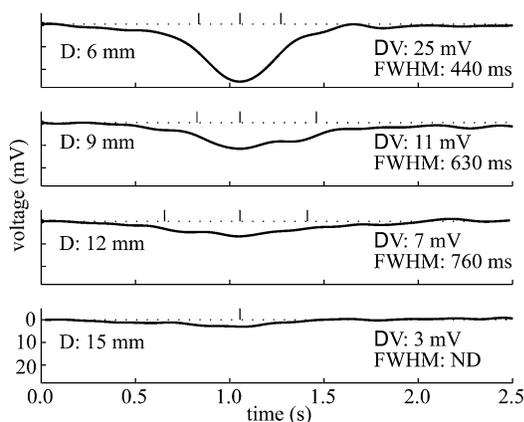
*Figure 2.* Voltage changes recorded from an individual array element as an object is scanned past the array at four different distances. The object was a 1 cm diameter plastic sphere. As the scan path was moved farther from the array, the peak amplitude of the perturbation decreased and the FWHM increased. The FWHM for the furthest scan was not determined (ND) because of the low signal amplitude.
