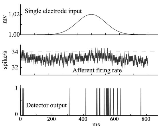
*Figure 3.* Illustration of a Gaussian voltage change similar to those measured being passed to a model of the electrosensory afferents. A neural detection algorithm based on a simple integrate-and-fire mechanism then processes the afferent signal.
