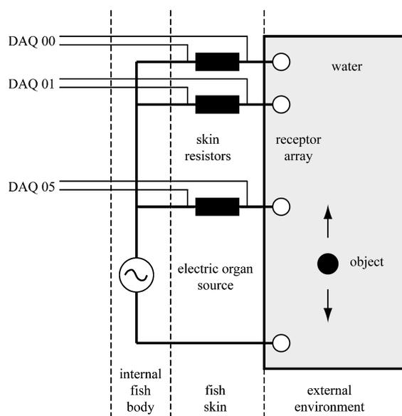
Figure 1. Schematic of the receptor array test setup. An electrolocation target was moved parallel to the submerged electrosensory array. Voltage signals, representing the transdermal potential experienced by each receptor, were recorded simultaneously from each channel as the target moved past the array.
