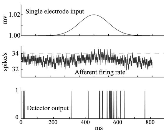
*Figure 3.* Illustration of a Gaussian voltage change similar to those measured being passed to a model of the electrosensory afferents. A neural detection algorithm based on a simple integrate-and-fire mechanism then processes the afferent signal.
