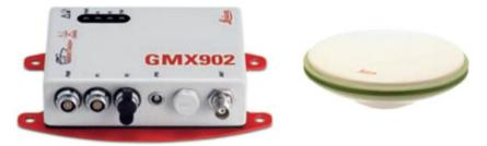
Figure 3. Leica GMX902 dual-frequency GPS receiver (left) and AX1202 antenna (right): 0.2 mm RMS accuracy, 2.4 W power consumption, and up to 20 Hz sampling rate [30].
